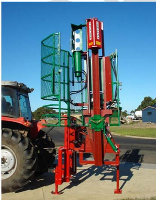
**Figure 7:** Tractor mounted post driver
