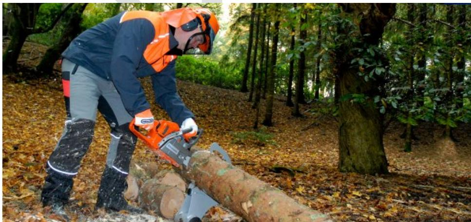
**Figure 1:** Chainsaw operator wearing PPE.
