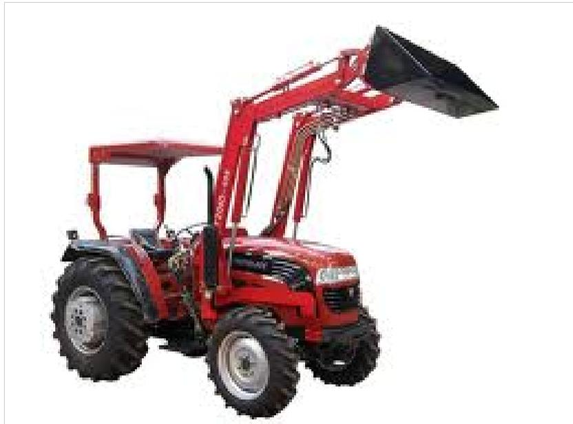
**Figure 6:** Tractor fitted with a FEL attachment
